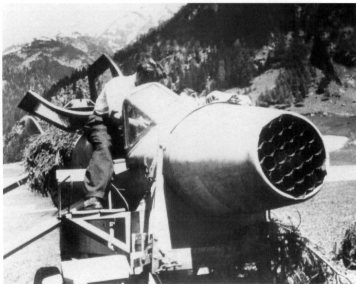
Production Ba 349 A Natter discovered by American forces in the Alpine region of Germany. The aircraft is equipped with launch tubes for 24 Hs 217 air-to-air rockets.
