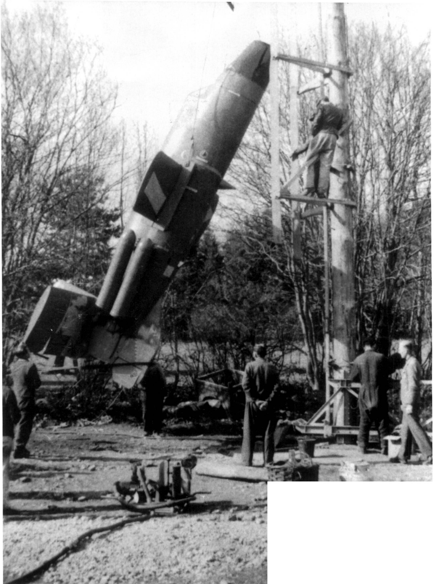
A provisional launch tower made of wood was used pending introduction of the production version made of steel. Unmanned test launches were conducted with this apparatus. Here one of the Bachem Ba 349 prototypes is seen being raised onto the tower.
