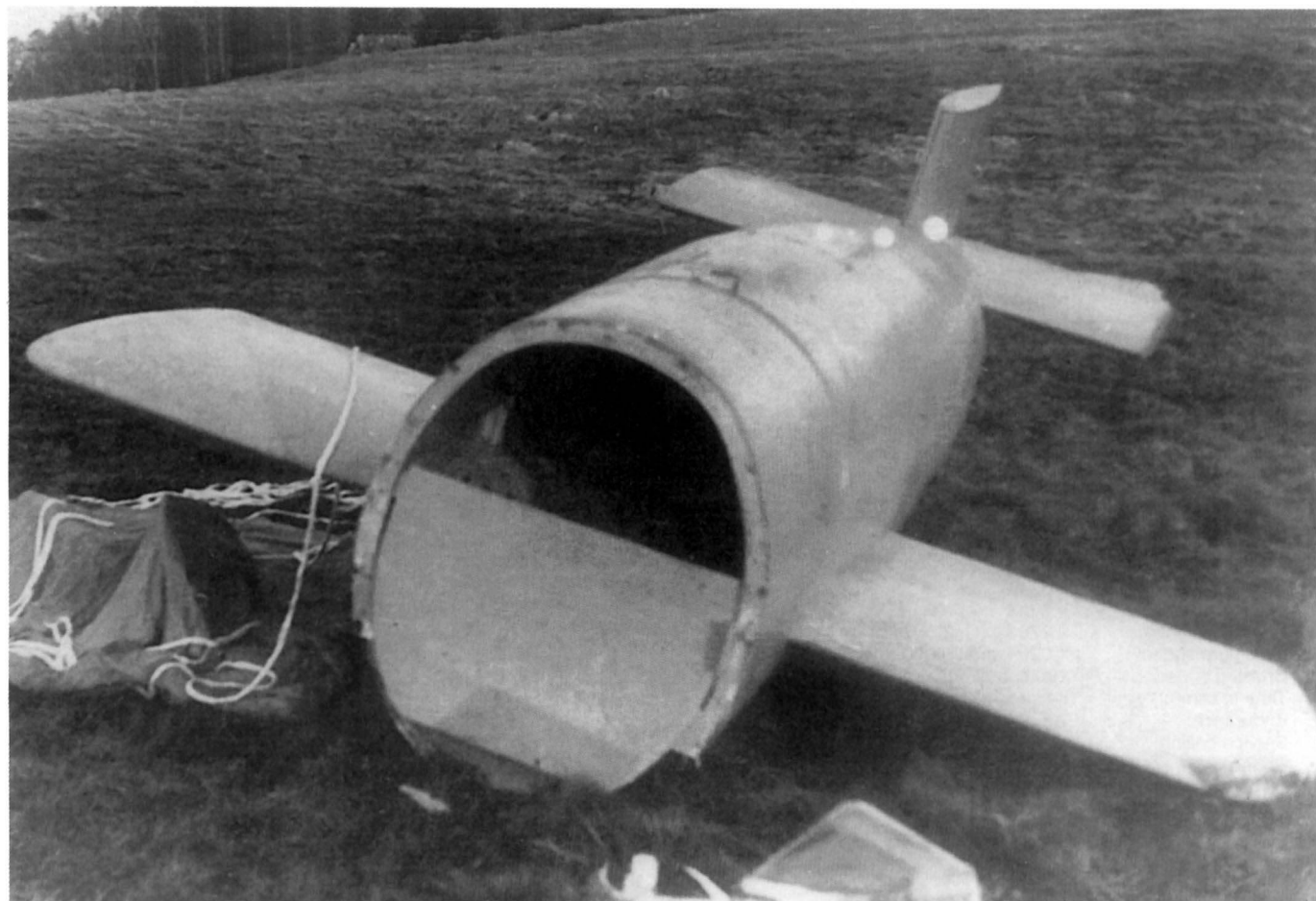
Natter aft section after separation of the nose and cockpit sections and return to earth by parachute.
