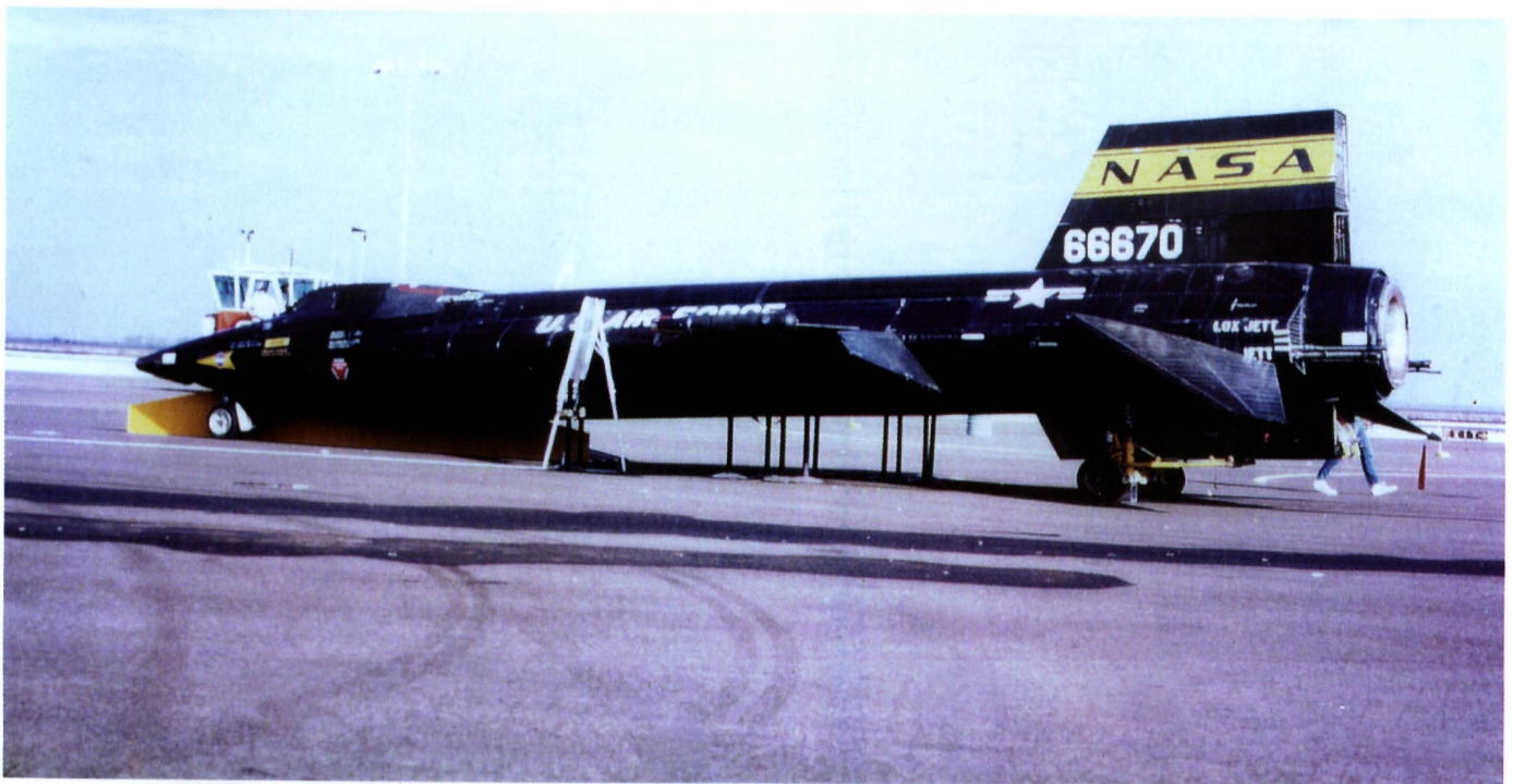
To date the X-15 represents the apex of rocket aircraft development, having achieved speeds on the order of Mach 6.7.
